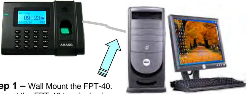
**Step 1** – Wall Mount the FPT-40. Connect the FPT-40 terminal using direct connection with included USB cable to host PC, or Ethernet cable for network connection. Plug the in the AC adapter to the FPT-40 and AC outlet and the FPT-40 terminal will power up.
